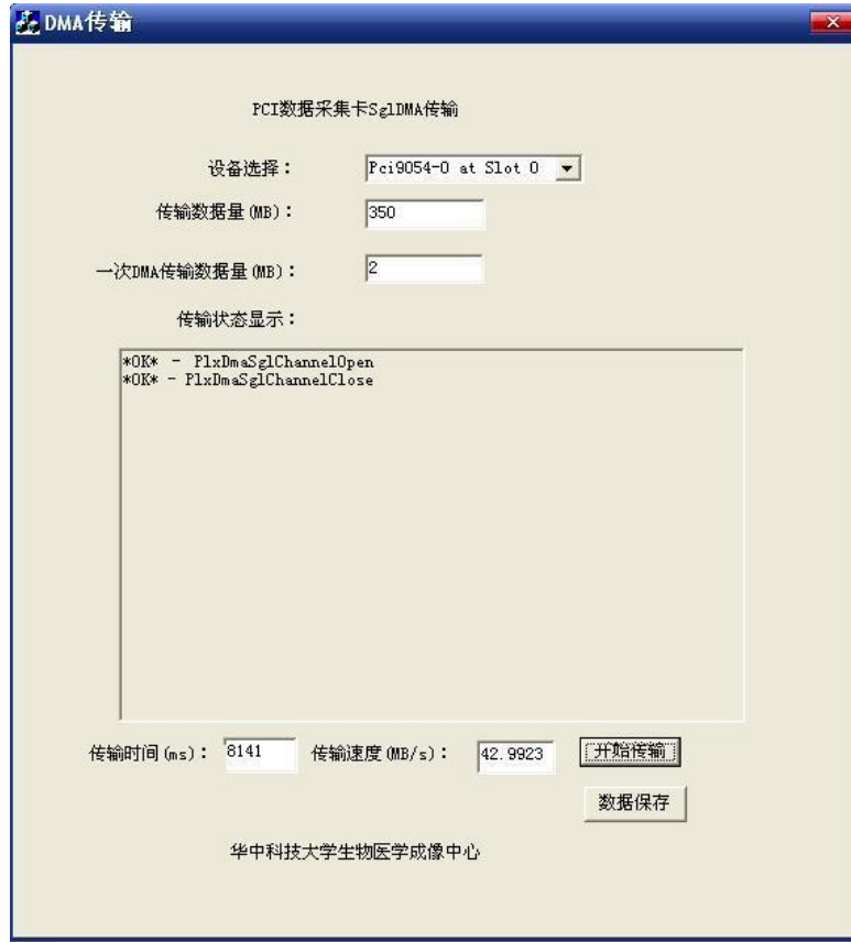
Figure 6. The dialog of the running Windows application program on our PCI board. The buffer for one time DMA transfer is 2MB. It takes 8141 ms to transfer 350MB data, corresponding to a data transfer rate of 43MB/s.
